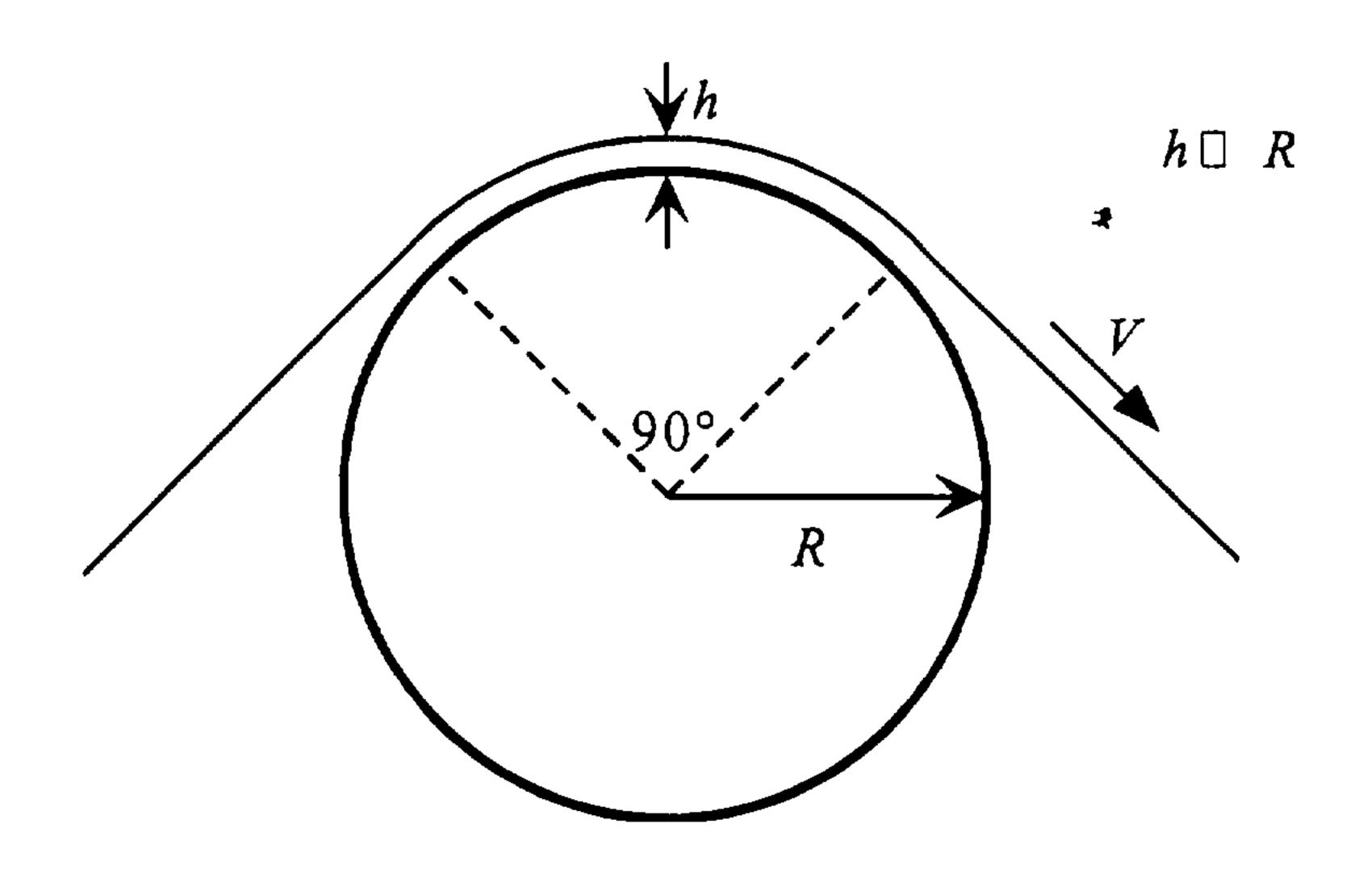
Now the roller is allowed to rotate about its center. The roller has a frictional torque  $T = C\omega$ , where C is a constant and  $\omega$  is the angular velocity of the roller. Find the force F required to move the sheet at the speed V. Find the angular velocity  $\omega$ , and comment on the limits when  $C \otimes 0$  and  $C \otimes \infty$ .
