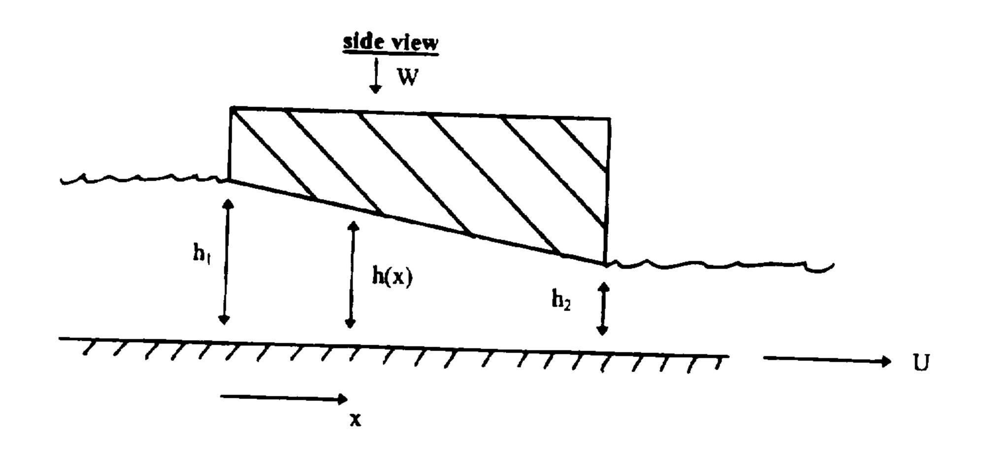
Consider the slider bearing, shown above. The width b is very small compared to length L, so the <u>narrow bearing</u> approximation can be used. Note that the slope of the lower slider surface,  $\frac{dh}{dx} = h'$ , is a constant.
