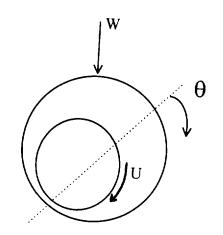
Consider a journal bearing of radius R, length L, clearance C and eccentricity ratio  $\epsilon$ . The surface speed is U and the viscosity is  $\mu$ .
