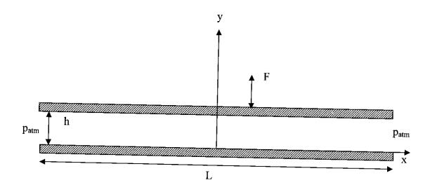
We would like to study squeeze film effects in a liquid (constant viscosity  $\mu$  and density  $\rho$ ) using the apparatus shown above. The liquid is contained between two plates of length L in the x-direction and very long in the z-direction (out of the paper). A time-dependent force is applied to the upper plate so that the film thickness h oscillates with time:
