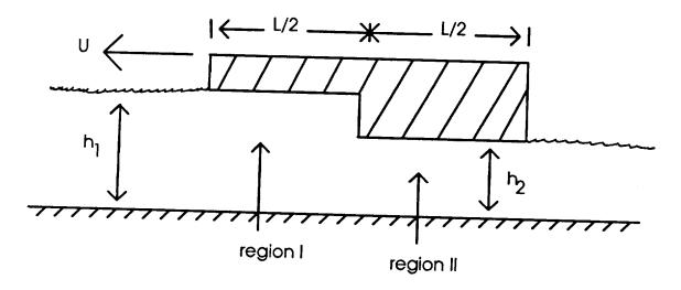
Consider the 2-dimensional step slider bearing shown above. The slider moves with speed U over a liquid film of constant density  $\rho$ , and constant viscosity  $\mu$ .
