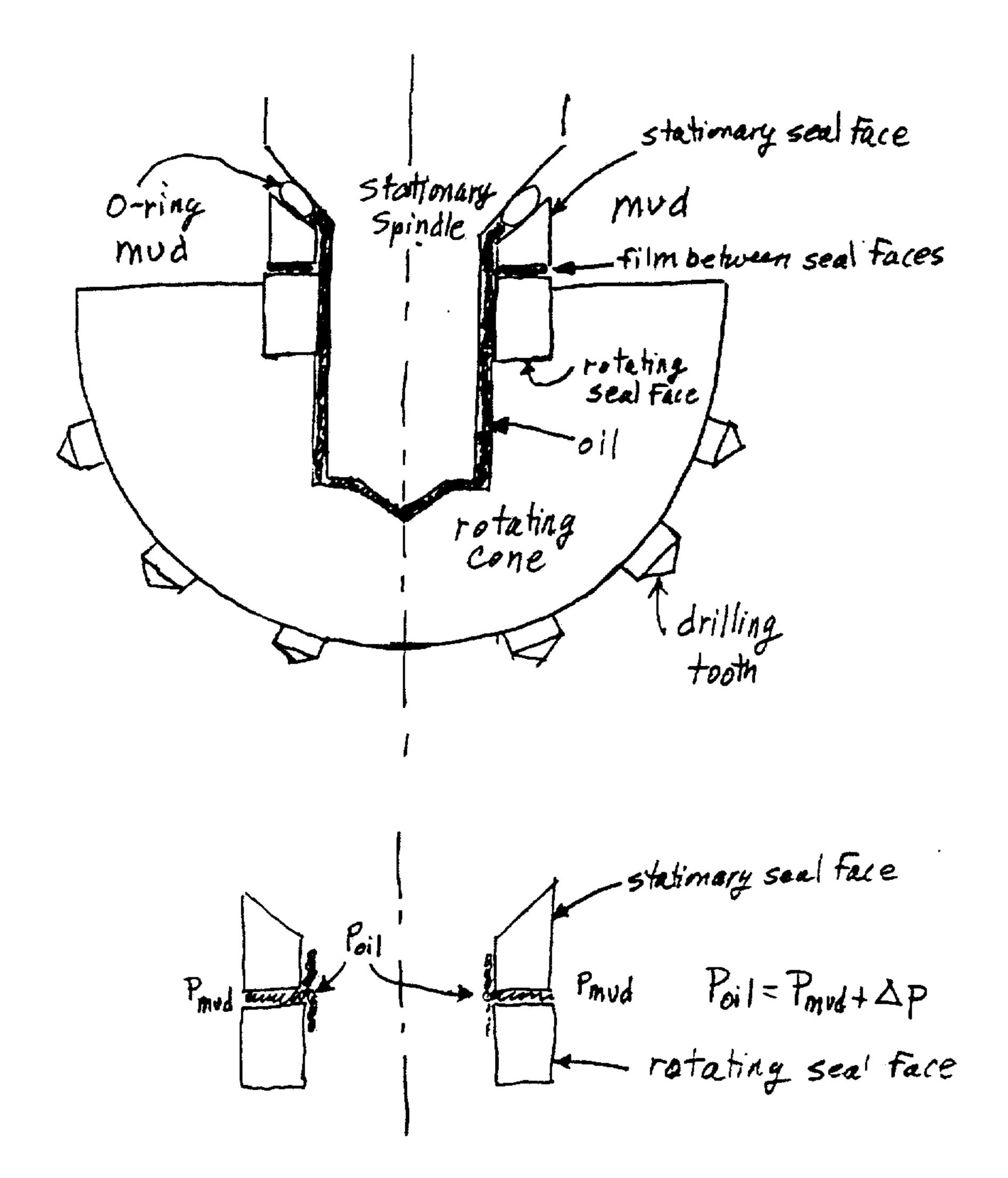
Consider an oil well drill bit, consisting of a rotating "cone" that holds the drilling teeth and a stationary spindle. The clearance between the spindle and the cone is filled with oil. Drilling mud (a viscous, abrasive liquid) fills the oil well outside of the cone and spindle.
