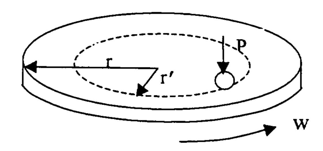
a. Under light loads and with smooth, non-adhering surfaces, the contact may be assumed to be Hertzian. Neglecting the roll of friction, draw a schematic diagram of the pin/disk cross section indicating the Hertzian contact zone whose radius is given by
