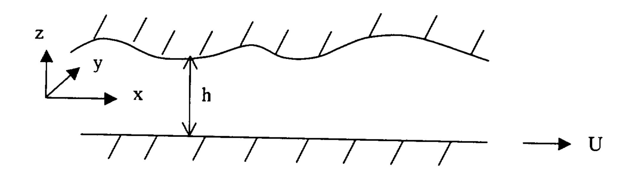
Consider the flow of a liquid lubricant between two surfaces separated by a distance h(x,y), with the lower flat surface moving in the x-direction with speed U, as shown above.
