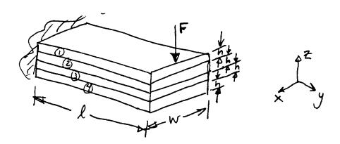
a. Suppose you don't know whether the layers are intimately bonded or are allowed to slide relative to each other. Can you make limiting assumptions and estimate an upper and lower bound of the force F required to produce a given (small) displacement  $\delta$  at the end of the beam? Show all work.
