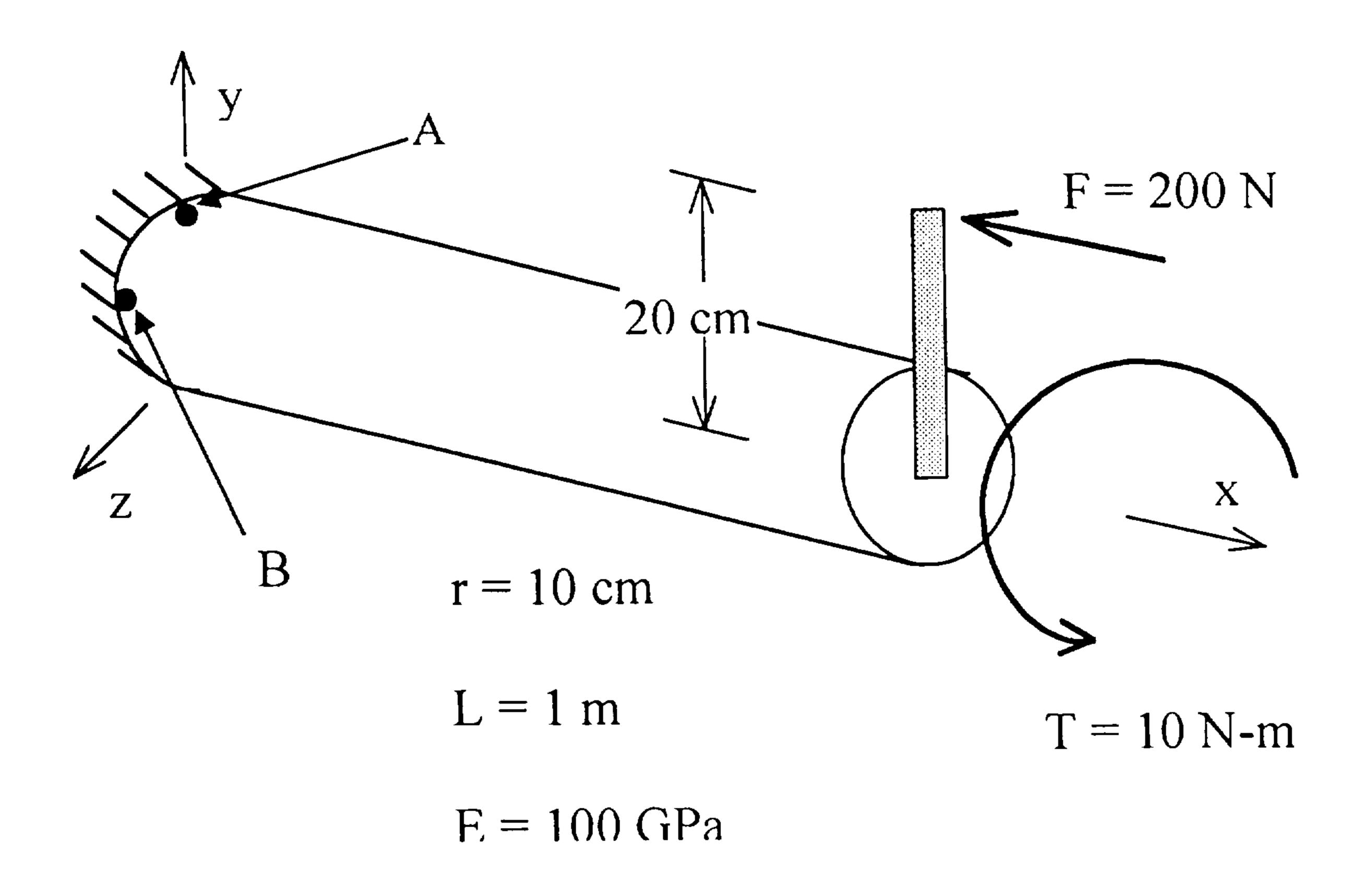
Consider the rod (1m long, 10cm radius) welded to the wall as shown above. A torque of 10 N-m is applied to the right end and a force of 200 N is applied to a bar attached to the right end.
