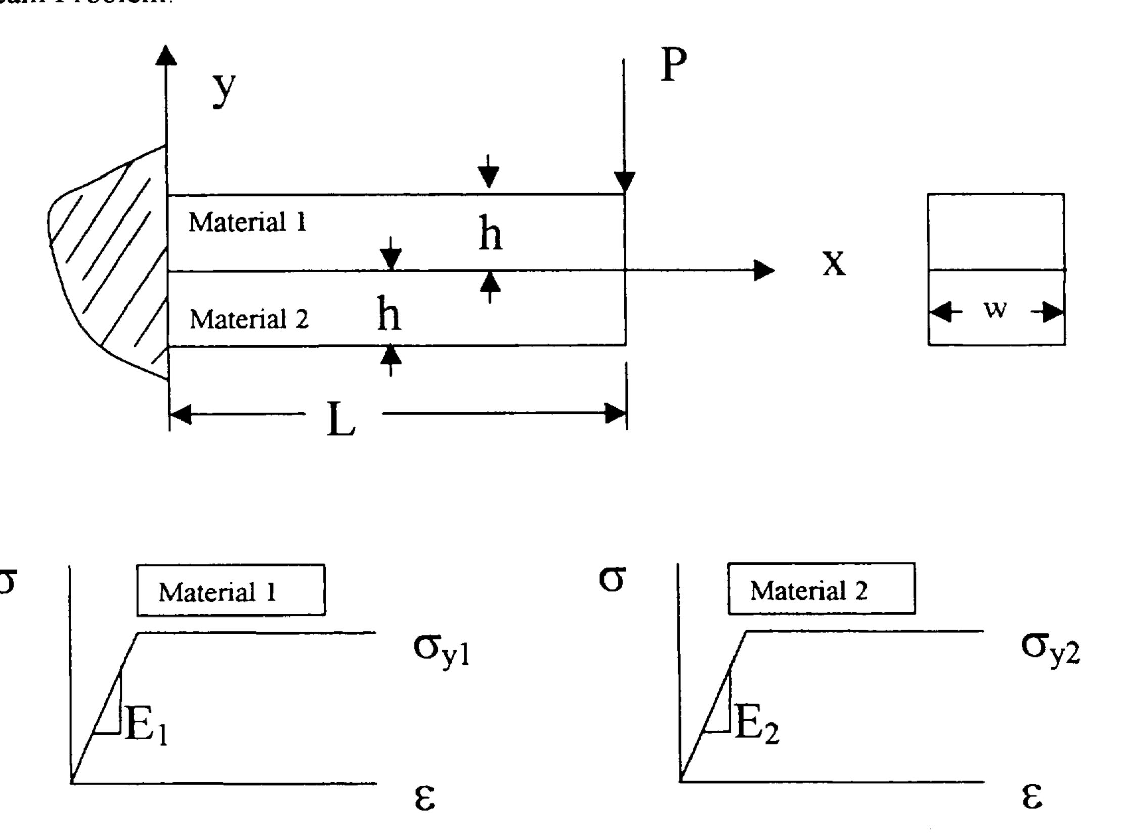
The bi-material cantilever beam above is subjected to the loading shown. Neglect transverse shear and use simple beam theory. Also, assume that tension and compression stress-strain behavior is symmetric.
