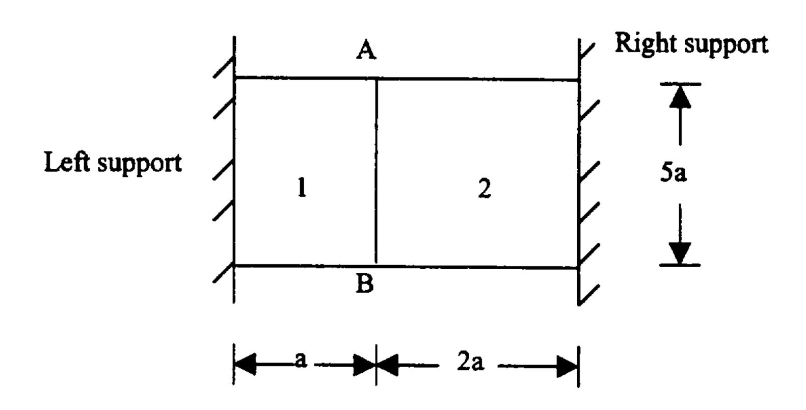
Problem 4: The bi-material cantilever beam below is subjected to loading as shown. Neglect transverse shear and use simple beam theory. The stress-strain curves for both materials 1 and 2 are shown given. Material 1 has symmetric yielding behavior in tension and compression, while Material 2 has twice the yield strength in compression compared to tension. Note that  $\sigma_{yT1} = 2\sigma_{yT2}$ . The Young's modulus of Material 2 is equal to that of Material 1,  $E_1 = E_2$ .
