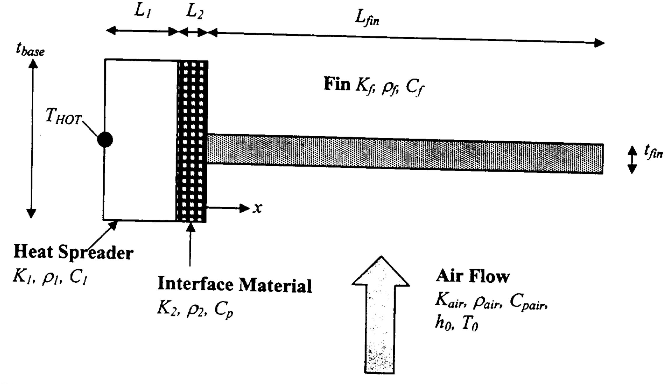
There are three materials in the system: two for the base and one for the fin. The thermal properties of the system are given in the figure.
