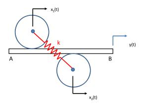
a) Find the linearized equations of motion using the coordinates  $x_1$  and  $x_2$ .
