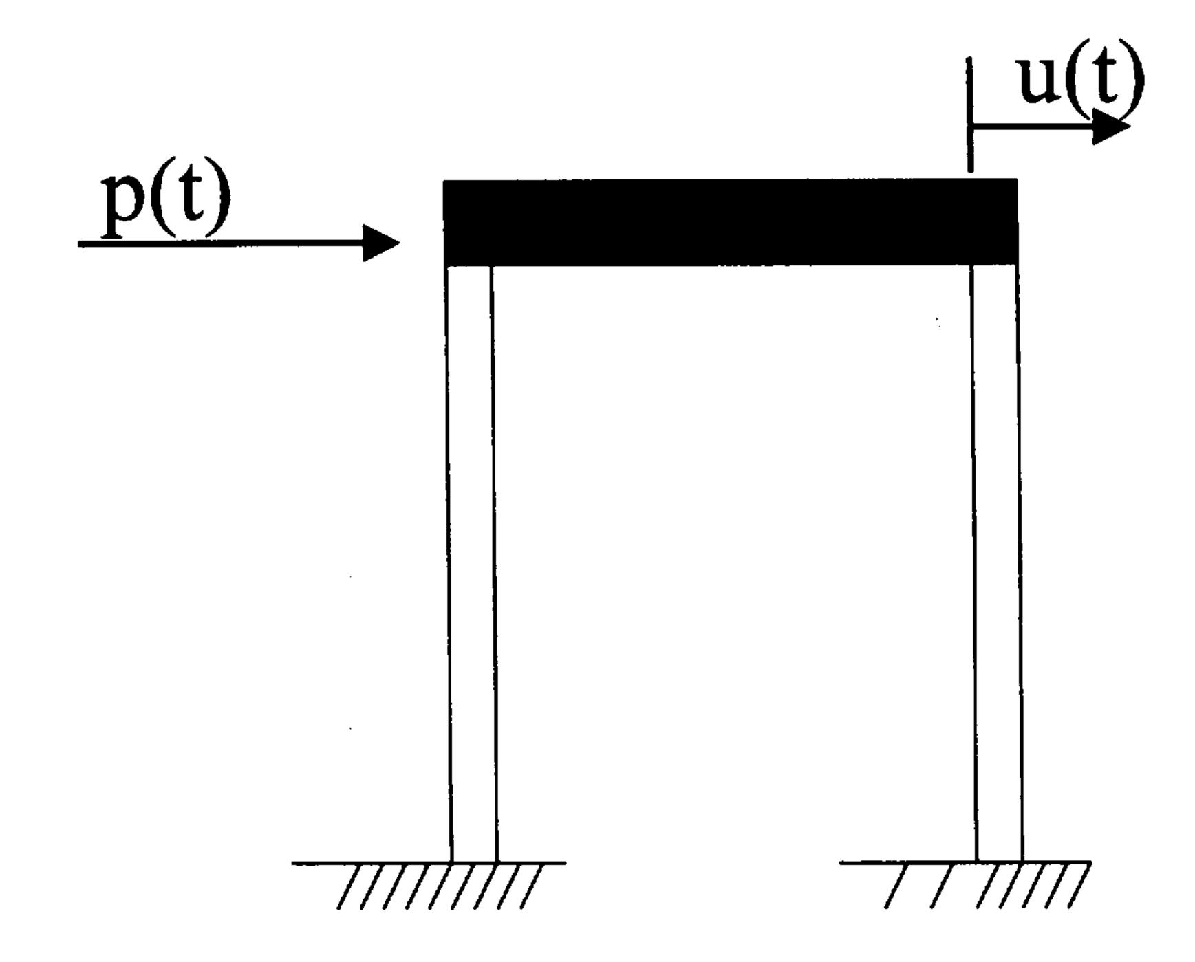
The above building frame is anchored at the rigid base and is subjected to a wind force p(t). In the above figure, m is the building mass, u(t) the lateral displacement of the mass and k/2 the lateral stiffness of each of the columns. The equation of motion can be approximated by
