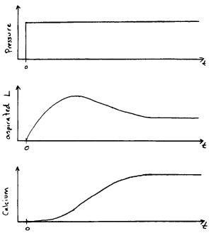
Part A) Wiesner et al. (PNAS, 1997) published a model of shear induced calcium influx in endothelial cells. These cells were exposed to fluid shear stress induced in one dimension in a flow chamber. Their model of the stretch-induced influx of calcium
