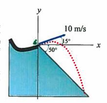
(a) Develop a projectile equation and determine the distance from the takeoff ramp to where the ski jumper lands, measured along the sloped surface direction.
