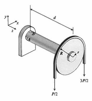
The shaft shown in the figure above is driven by a belt. The tension in the belt on the tight side is 3P/2 and the tension on the slack side is P/2.
